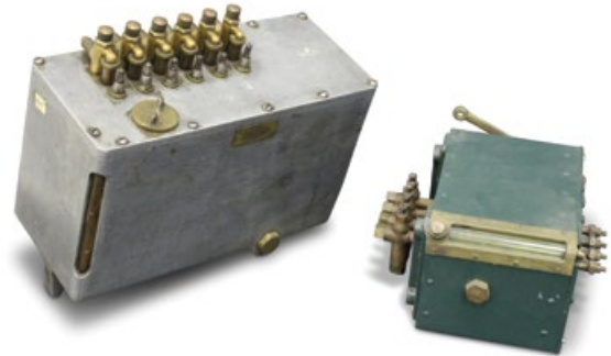
133 Pair of Firewall-Mounted Oilers
